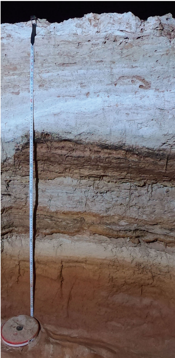
Figure 3. Geotrench 2 eastern profile exemplifying uncemented sediment sequences exposed in FB1 and FB2 geotrenches.
